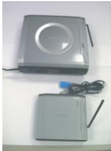
Figure 1-1 Wireless transm. receiver cabinets
